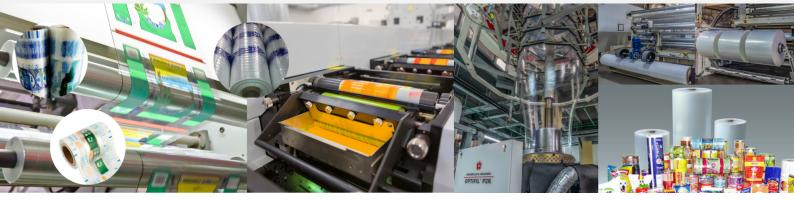
Ashkal PS40 is a unique PE formulation that prepares the surface of the film for high-speed rotogravure and Flexo printing process. The film is compatible with conventional polyurethane and Vinyl Inks systems. The specially designed mechanical and surface properties film including machine direction elongation and overall stiffness, allow conventional printing systems to run the film for all kinds of surface or reverse printing jobs.
